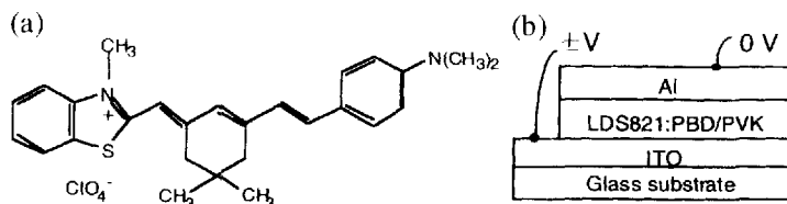
FIGURE 1 The structure of LD S821 (a) and the LEDs fabricated in this study.
